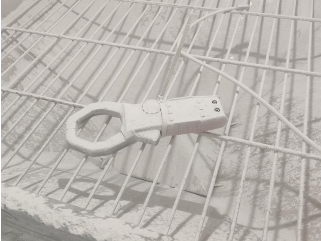
Photo 1 – During IP5X testing
