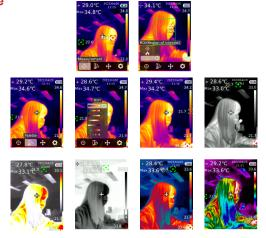
In the main interface, press the SET button to open the main menu. Press the Left/ Right button to select "Palette", and press the SET button to open its submenu. Press the Up/ Down button to select a palette. Press the SET button to use the selected palette. Press the Return button to return to the previous interface.
