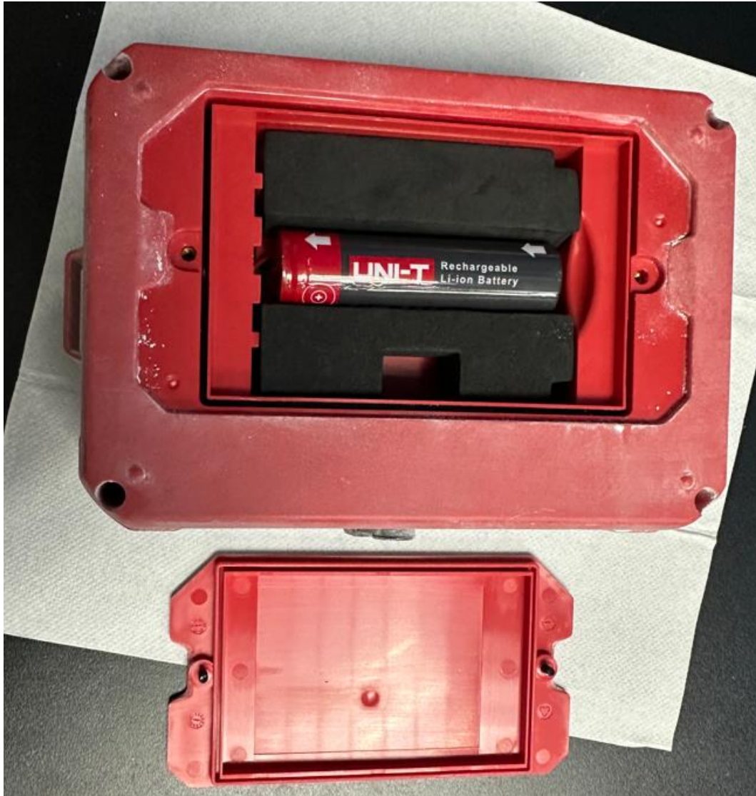
Photo 5 - Internal view after IP5X test
