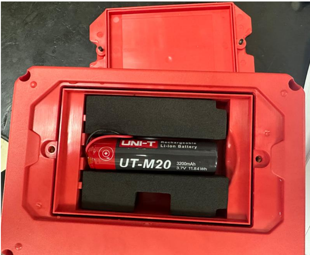
Photo 4 - Internal view after IPX4 test
