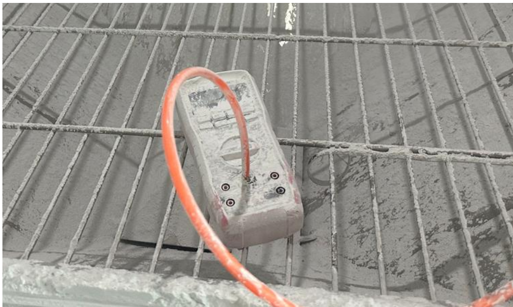
Photo 2 - Product during IP6X test
