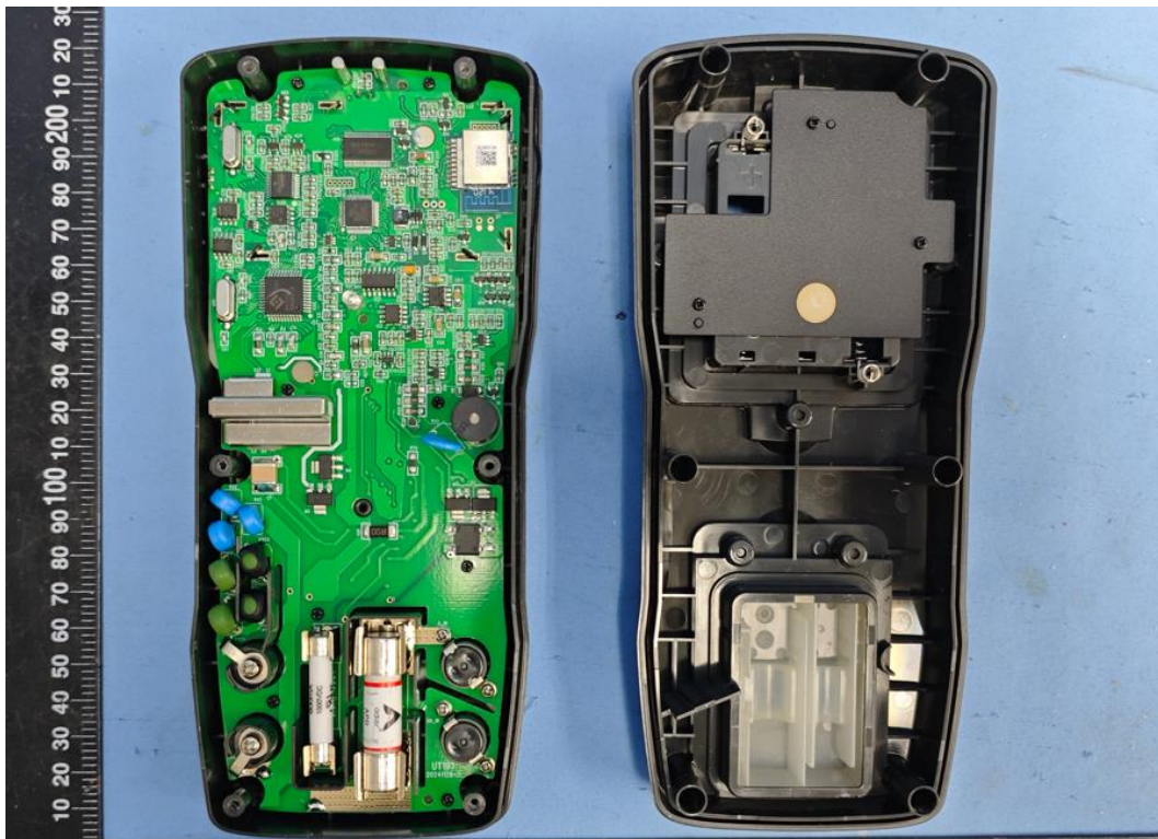
Photo 3 - Product after IP6X test
