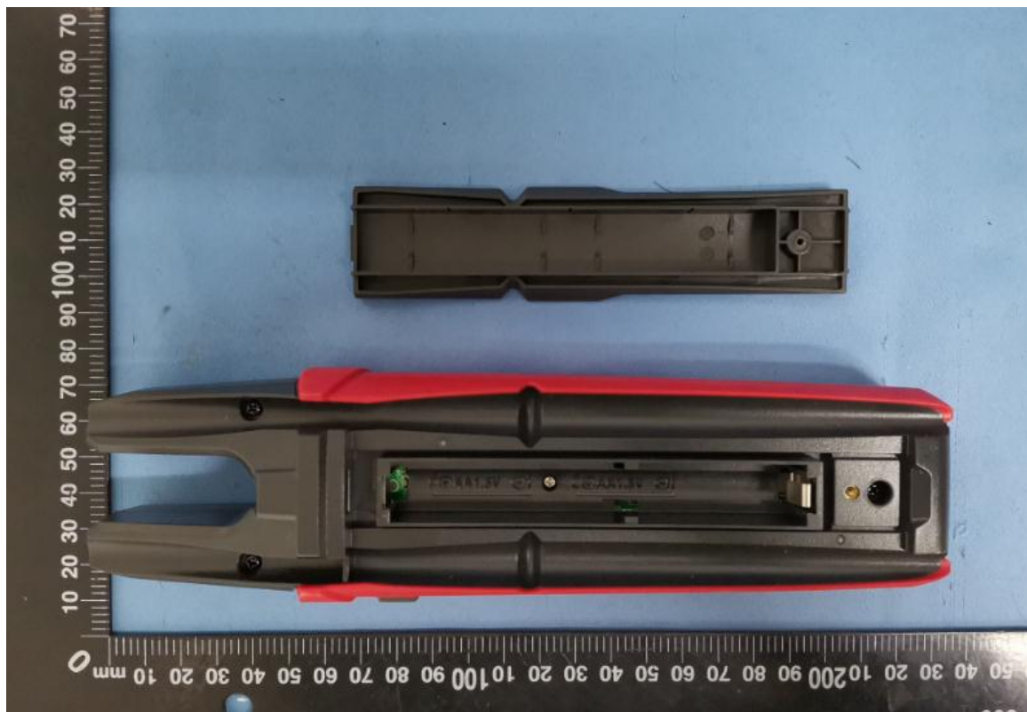
Photo 3 – Battery box view
